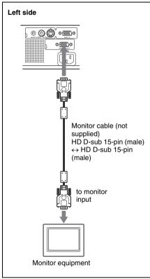
\* This projector is not guaranteed for connecting more than 2 monitors in loopthrough connection.
